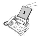
Be sure to load the paper so that printing takes place on the **print** side of the paper. Printing on the reverse side will result in poor print quality.
